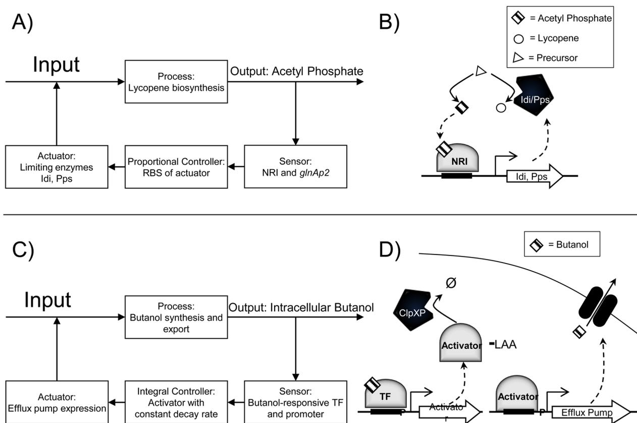
**Figure 4. Block diagrams and molecular mechanisms of feedback controller designs**
